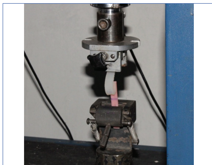
[Table/Fig-4]: Prepared acrylic and silicone specimen placed in the universal testing machine for the peel bond test.
